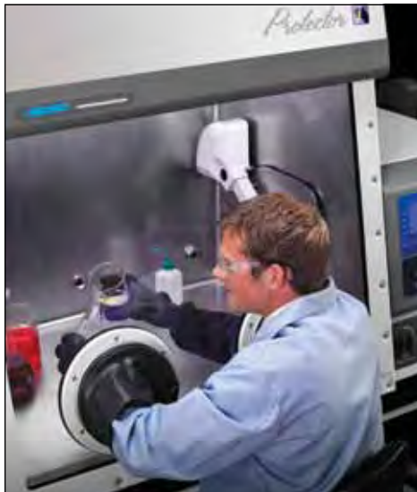
Protector Controlled Atmosphere Glove Boxes create ultra low oxygen and moisture conditions inside the chamber for applications involving sensitive materials.
