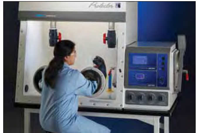
Protector Combination Glove Boxes have features of both filtered ventilated and controlled atmosphere glove boxes. Two internal valves allow the box to be converted from filtered mode to controlled atmosphere.
